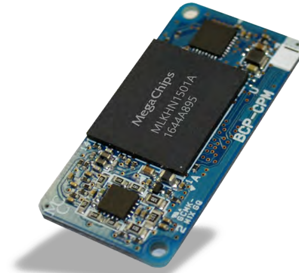
Complete HD-PLC Compact Circuit Design (15mm x 40mm)
