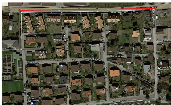
This PLC installation covered 342m from transformer station to distribution cabinet. Throughput over this connection is about 20Mbps.
